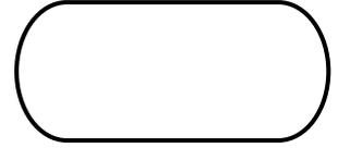
Finally, an oval is also used to represent the end. It is a termination point. This symbol is used at all termination points, not just the very end.
